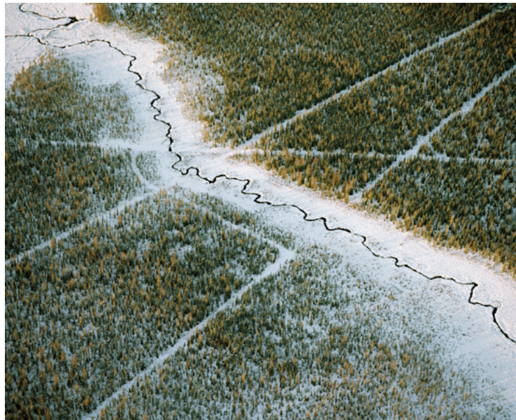
Figure 4. Cut Lines - Aerial view of seismic cutting through boreal forest near Edson, Alberta.
